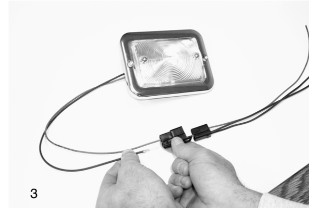
Photo 3 shows the finishing of a parking lamp pigtail assembly using terminals N and connector L. The pigtails will connect to the 500432 front light harness using terminals H or J along with connector M as shown on page 8 of this instruction set.
