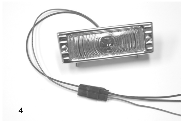
Photo 4 shows the completed pigtail assembly as it looks once plugged into the 500432 front light harness kit.
