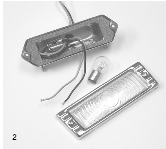
Photo 2 shows the same method as photo 1, but applies to a dual wire parking lamp (brown and blue wires). You must re-use your original 2 hole wafer insert, as it is NOT included in this kit.
