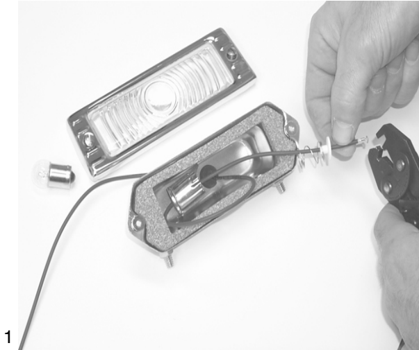
Photo 1 shows the spring R and wafer P installed onto the brown wire prior to rivet Q being crimped onto the brown wire.
